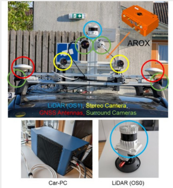
Figure 1: Experimental vehicle set-up. The main localization sensors include an Ouster OS1-128 LiDAR (blue), two forward-looking Basler stereo cameras (yellow), and dual GNSS antennas (red) for precise attitude determination. Surround cameras (green) and an additional OS0-128 LiDAR at the front are used primarily for object detection. Onboard processing is performed by a Car PC (bottom left) running computer vision algorithms and the ANavS AROX system (orange, top right), which hosts the tightly coupled GNSS/IMU filter and the multi-sensor fusion algorithm.
